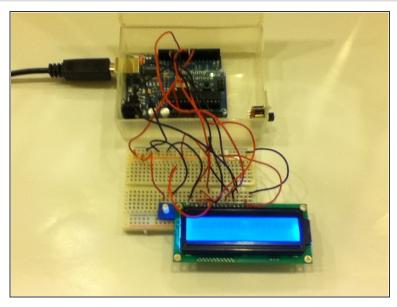
Then, wire up the LCD screen according to the <u>instructions</u> on the Maker Shed site.
